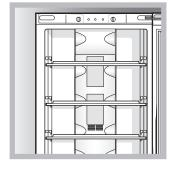
This is recognisable by air ducts located on the back walls of each compartment. The No Frost system circulates cold air continuously to collect humidity and prevent ice and frost formation. The system maintains an optimal humidity level in the compartment,
